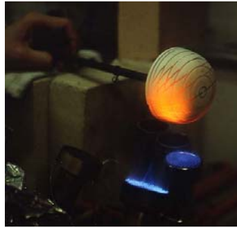
Heating the Core. The Design is Marked on the Core
