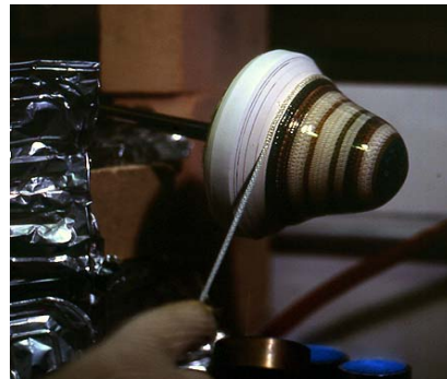
The Canes Applied concentrically on the side of the core of vessel M7
