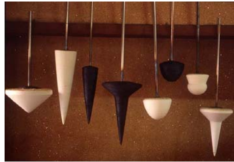
The Cores Prepared for various vessels. They are made of steel wool & clay Held by steel rods
